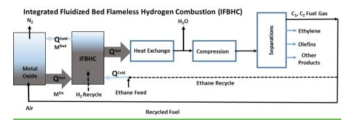
Rather than cracking ethane, oxygen transfer agents (OTAs) are used to convert ethane to ethylene via the selective combustion of hydrogen in the presence of hydrocarbon feed and products.
